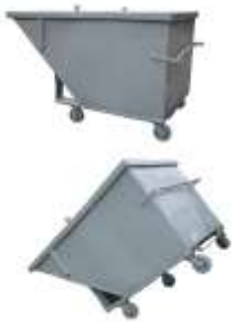
44" x 68" x 43" manual tilt truck 2000# capacity, 6" casters – 2 rigid/2 swivel, painted gray
